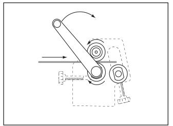
Figure 19. Feeding the workpiece.
